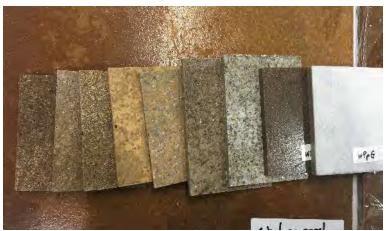
Waste engineered timber coming from demolition sites and remanufactured panels from UNSW research.
