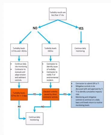
Figure 1: Turbidity Management Framework. (Source: SHIS Construction Water Quality Management Framework, TI 2015)
