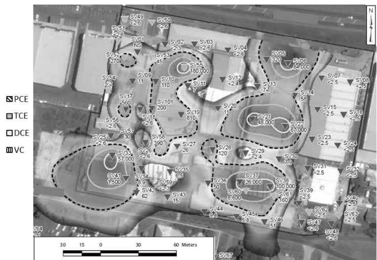
Figure 1. Typical PCE, TCE/DCE and VC dominated soil-vapour results, showing variability in contaminant type/degradation; and example isopleth plot for TCE in soil-vapour (dotted line represents adopted criterion, units in µg/m 3 ) (after SiREM 2015)
