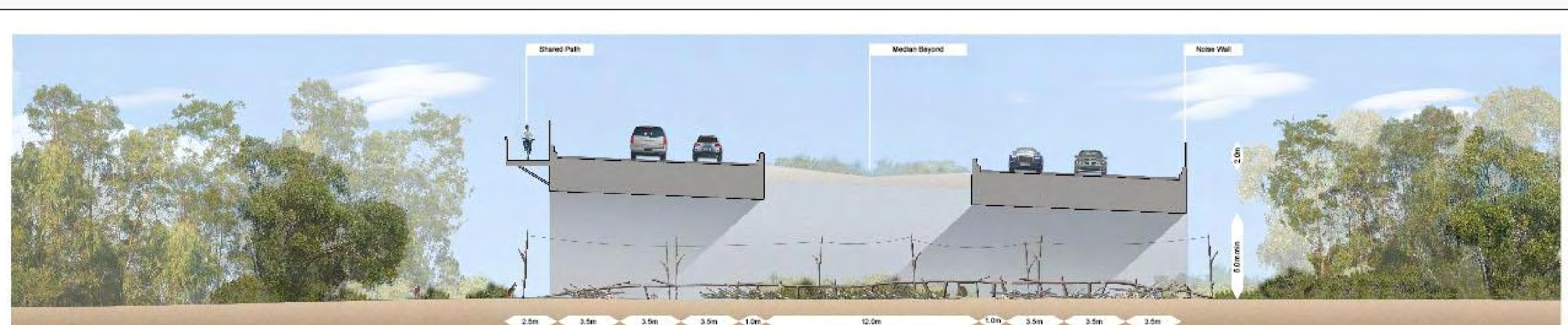
Figure 4.1 Cross Section at Fauna Crossing
